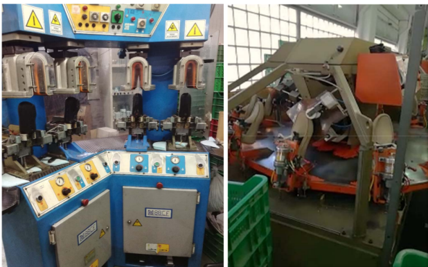
Figure 6 - Rear parts forming machine (Talonadora) and front parts forming machine (Rotostir).
