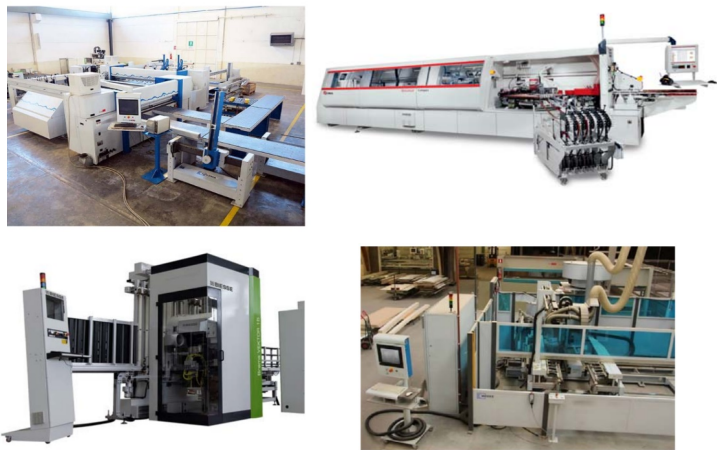
Figure 8 - Podium machines (cutting - HOLZMA-HKL, edge bander - IMA and drilling - VEKTOR 15 and MAW ABS 100).
