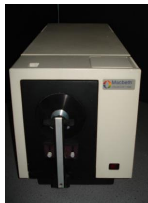
Figure 11: “Macbeth Color-Eye 7000” Spectrophotometry
