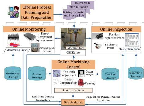
Fig. 4. Framework of the integrated monitoring system [65]
