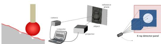
Fig. 3. Methods of quality inspection: (a). tactile; (b). optical; (c). X-ray
